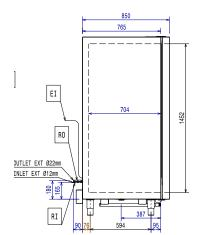
Drain Electrical inlet (power) RΩ Refrigerant Outlet
